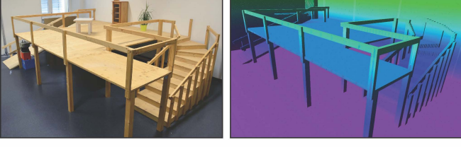
Fig. 2. Photograph of the environment in which we carried out the experiments and the corresponding map constructed with a CAD software. The map contains only the static parts of the environment.
